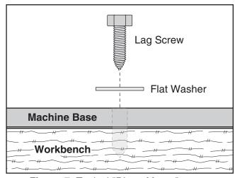
Figure 7. Typical "Direct Mount" setup.
